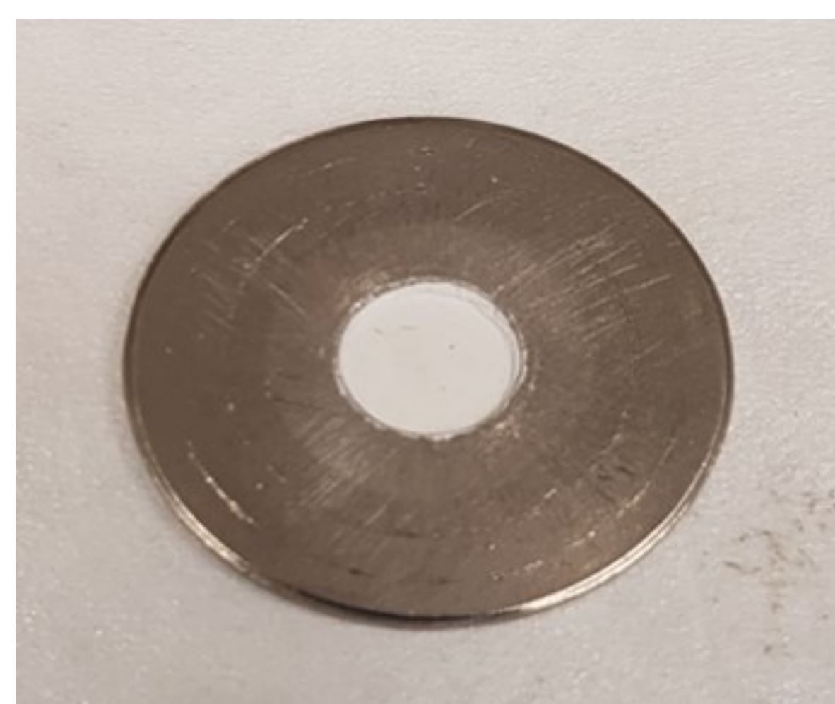
Image 1. ^{86}\text{Sr} ]SrO powder pressed into cavity of Niobium target disk
