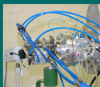
COSTIS target station connected with the external beam of the IBA cyclotron
