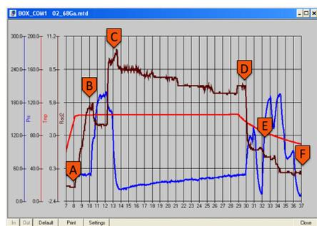
**Figure 3.** Chart of [<sup>68</sup>Ga]DOTA-NOC synthesis. A: generator elution/SCX retention; B: SCX elution; C: Start reaction; D: C18 purification; E: C18 elution; F: EOS.
