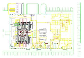
70000 Square foot ( $6500 \text{ m}^2$ ) building is located in the town of Noblesville, approximately 20 miles (32 km) north-east from Indianapolis. Approximately 40% of the building is occupied by a cyclotron and associated support equipment, separated into a restricted zone. The rest is used for laboratory and office space and reserved for future expansion.
