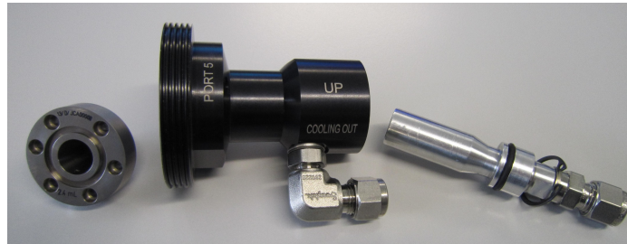
New conical design #: Niobium insert, target body, water diffuser
