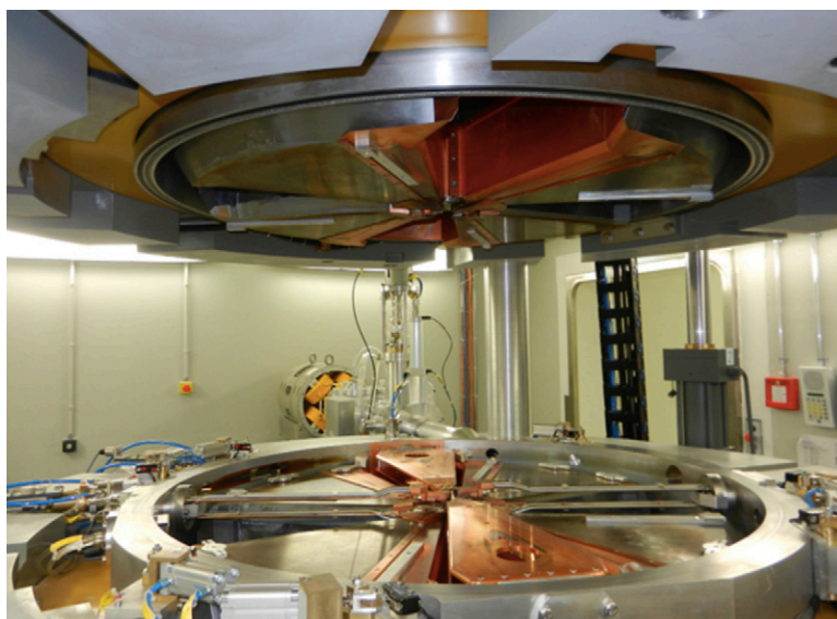
Figure 1. The Bern cyclotron opened during commissioning. The part of the BTL located in the cyclotron bunker is visible, pointing towards the wall separating the two bunkers.
