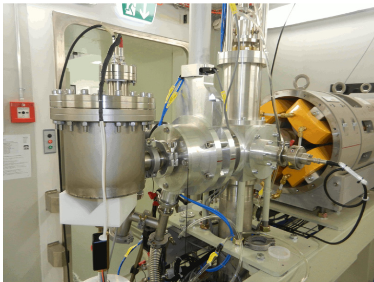
Figure 3. The high sensitivity Faraday cup installed at the end of the BTL for low current performance studies.
