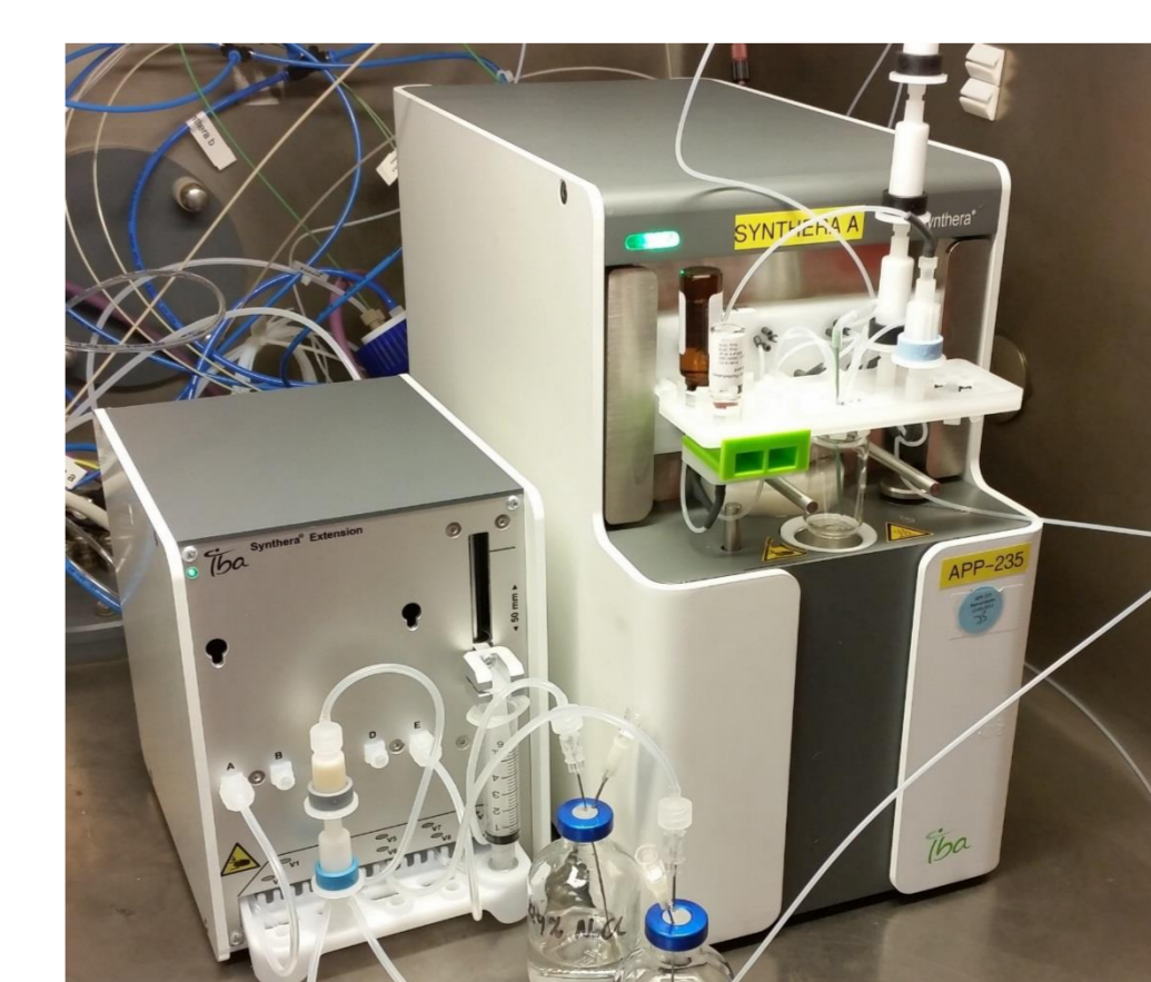
Synthera® Synthesizer and Extension set-up at BV cyclotron for the optimization of 18 F-FCH process.
