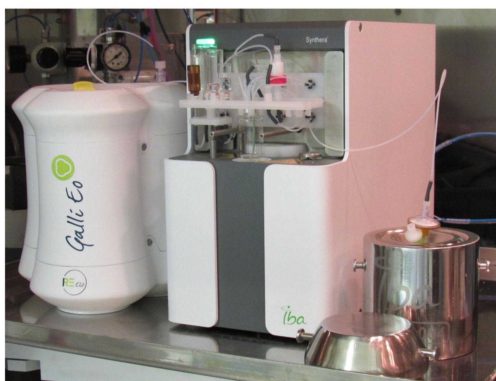
Set-up in a standard hot cell: Synthera ® synthesizer combined with IRE Galli Eo ™ ^{68}\text{Ge}/^{68}\text{Ga} generator
