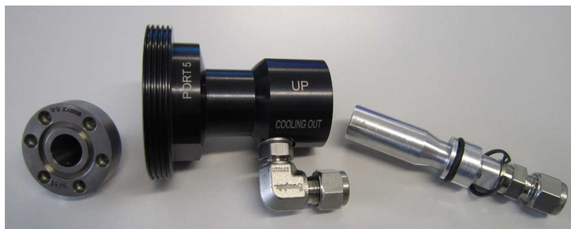
Figure 9: New conical design [3]: Niobium insert, target body, one piece water diffuser
